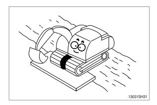
When working on soft ground, place mats or wood boards on the ground to prevent the machine sinking.
